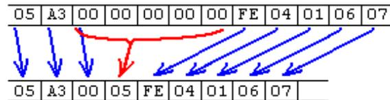
**Figure 2. Modified RLE compression – compressing only zeros.**
