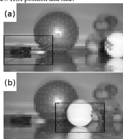
Fig. 1. AV-based analysis of an image with a ROI. The inside of the ROI rectangle is being processed, while the outside of ROI is compressed with quality good enough to notice new objects. The vision system was examining the red car (a), when the tennis ball has entered the scene (b). While the ball is a relatively new object, it attracts the system’s attention.
