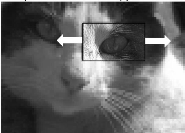
Fig. 3. Step-by-step high-level pattern spatial coexistence verification. The vision system recognizes an eye and then the algorithm “decides” to check if there is another eye in the image, to prove that the object should be recognized as a face. A face may be a part of a human or an animal; it may contain some characteristic features.
