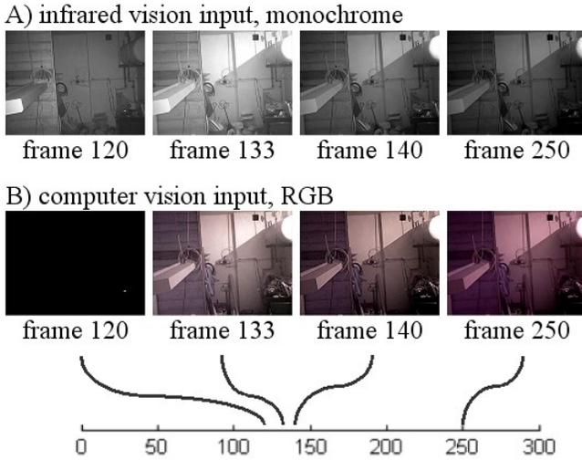
Fig. 2. The exemplary visual data input: darkness (frame 1..127) and with a dim light turned on (frame 128..288). Frames 128..140 are too bright due to the automatic white balance feature.
