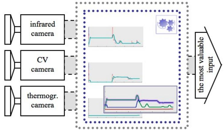
Fig. 4. The Policy-based Input Switching system's wrapper for automatic data input quality evaluation and selection. The policy (depicted as the dotted rectangle) can be replaced depending on circumstances and the working environment.
