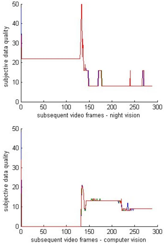
Fig. 1. Comparison of two acquisition subsystems, showing data quality during a change of lighting in the scene.
