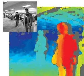
Figure 13. Depth image from a Stereovision camera [20].
