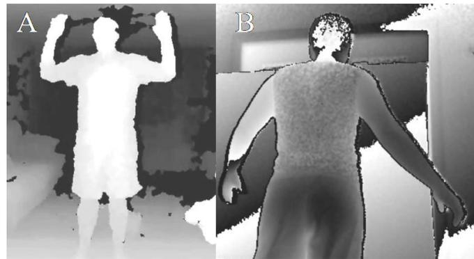
Figure 4. Depth map comparison: Kinect (A) [7] and Kinect 2 (B) [8].
