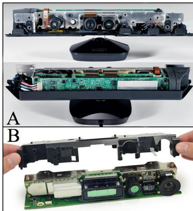
Figure 3. Inside view of the Kinect Sensor (A) [4] and the Kinect Sensor 2 (B) [5].
