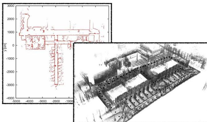
Figure 9. Maps generated using Laser Range Finder Scanners. Left/back: exemplary 2D LRF Scanner map [14], right/front: exemplary 3D LRF Scanner map [google.com].
