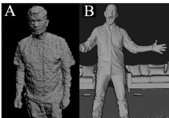
Figure 5. Point Cloud comparison: Kinect (A) [7] and Kinect 2 (B) [9].
