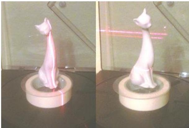
Figure 11. Home-made 3D Imaging Scanner. Left: vertical scanning mode (more useful one), right: horizontal scanning mode [own work].
