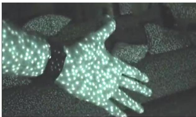
Figure 2. Infrared structured point cloud of Kinect Sensor [2].
