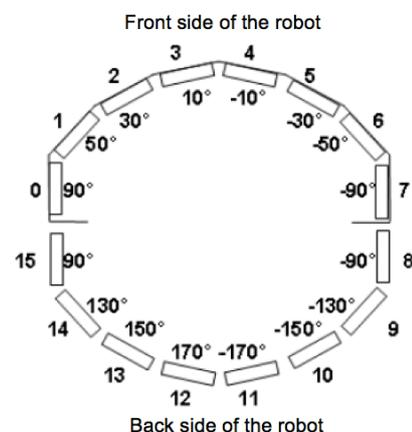
Figure 7. Placement of sonar sensors in a Sonar Ring of a mobile robot.
