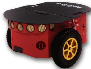
Figure 6. Pioneer 3DX mobile robot with Sonar Ring [10].
