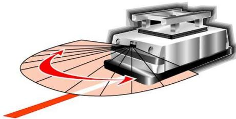
Figure 8. Laser Range Finder 2D Scanner on a mobile robot base [13].
